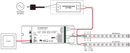
Note: please make sure the dial switches are at position for RGB+CCT mode as shown in above diagram.
