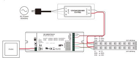
Note: please make sure the dial switches are at position for CCT mode as shown in above diagram.
