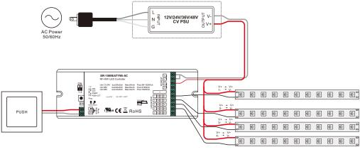
Note: please make sure the dial switches are at position for DIM mode as shown in above diagram.
